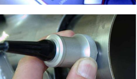
The ultrasonic thickness gauge is used to measure wall thickness, which is key information to calculate the exact inner pipe diameter.
