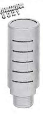
HFMA-Series high flow muffler features a 50 mesh, self-cleaning stainless steel screen, and combined with corrosion-resistant aluminum shell to create a highly efficient, ultra-quiet muffler designed with minimal back pressure.
