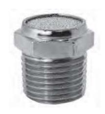
BV-Series low profile breather vents have many applications. They are most often used on single acting cylinders or valves to prevent dirt and foreign particles from entering ports open to the atmosphere. Common uses can also be found on vacuum relief or pressure equalization for gear boxes, crank cases, storage tanks or other vessels whenever pressure equalization is required.
