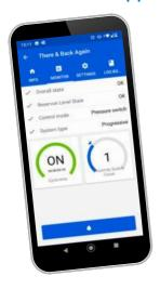
The app displays all SKF eLube devices within reach, monitors the lubrication status and indicates the system health at a glance.
